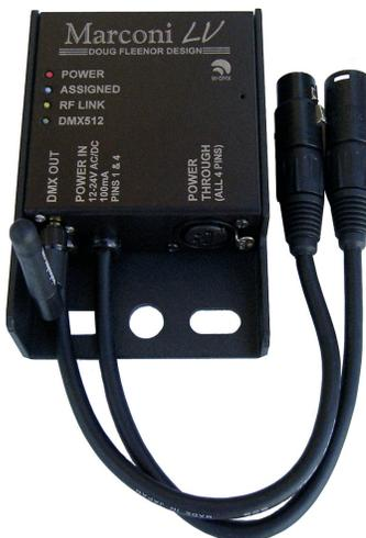
The Marconi "low voltage" (*Marconi LV*) is identical in performance to the *Marconi SP* but is powered by low voltage instead of line voltage and has only one DMX512 output. The *LV* is designed to mount to our *LED300* power supply but can be used with any 24V system that provides power on pins 1 and 4 of a four pin XLR (color scroller for example). The *LV* may also be powered by an optional external supply.
