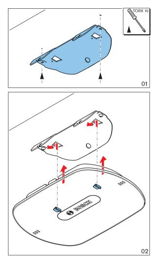
Figure 5.3: Mounting to a wall or ceiling
