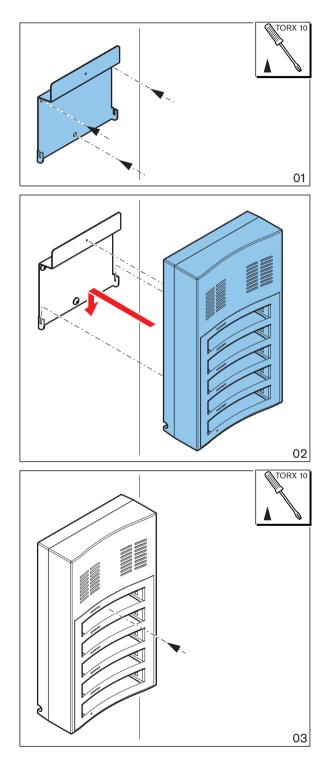
Figure 6.7: Installation to a wall
