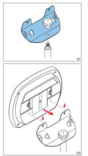
Figure 5.4: Mounting on a tripod floor stand
