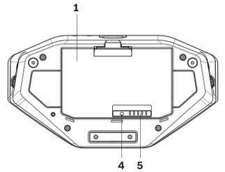
Figure 6.4: Wireless Device bottom view including Battery Pack
