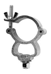
The Mini-Coupler is I" wide and fits from 1.65" OD to 2" OD Tube. The Mini-Coupler uses a  $3/8'' \times 3/4$ " long Grade 5 bolt with a Belleville washer and a Nyloc nut. The Mini-Coupler has a safe working load of 330 Pounds. (150 Kg)
